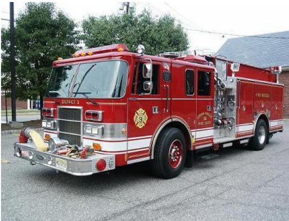
Cedar Knolls Engine 35 1995 Pierce Lance - 6 Man Cab Rescue truck - Jaws of Life, Holmatro, Hurst 1500 GPM Two Stage Waterous Pump 30 gal 3x3 foam
