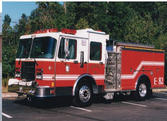
Whippany Engine 82 1995 Spartan/ US Tank – 6 man cab 500 Gallon Tank 1250 GPM Hale 2-stage pump
